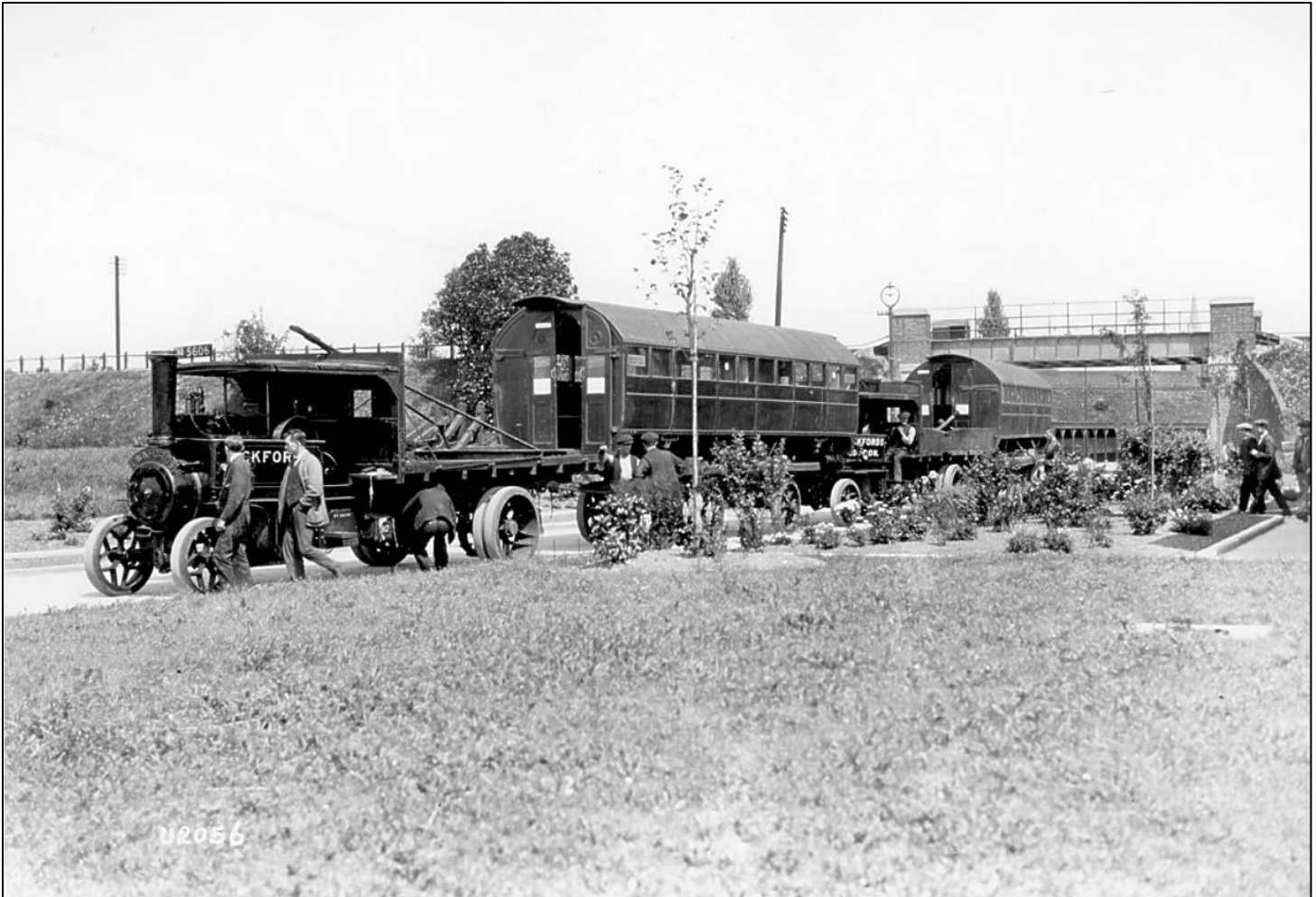
Figure 7: Two Hurst Nelson cars (minus bogies) being hauled by road into Acton Works in 1925. They were to become changing rooms for the new sports field being provided next to the works for District Railway employees. Source: Collection: B.R. Hardy,
